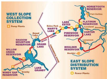
On the east slope, Broomfield’s water is stored in Carter Lake, located in the foothills west of Berthoud. From there, it is transported to Broomfield’s treatment facility via a 33-mile pipeline. The pipeline is part of the Southern Water Supply Project, also operated by the NCWCD. In addition to supplying water for Broomfield, this project serves a number of Front Range communities.
